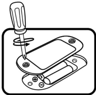
3. Install 2 new 'AAA' (AM-4/LR03) batteries following the diagram inside the battery box. (The use of new alkaline batteries is recommended for maximum performance.)
