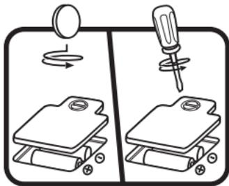
4. Replace the battery cover and tighten the screw to secure.
