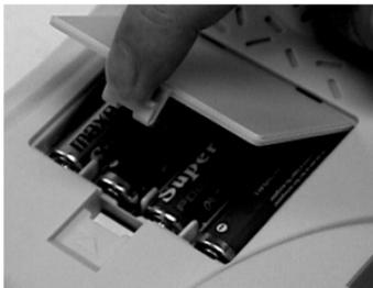
**Notice :** If you have been using the computer for a year, it's better to change the backup batteries. Because when the backup batteries run out, the computer can't power on and off normally. Only batteries of the same and equivalent type as recommended are to be used.
