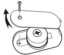
**NOTE:** While replacing the backup battery, the 4 “AA” size batteries must be kept in the unit, or the **Compact Notebook** should be plugged into the wall outlet with a 9V adaptor. Otherwise, you will lose all the information stored in the following applications: Phone Book, Music Composer, Personal Profile, and Progress Report.
