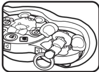
2. Push the pins on the soft bumper into the main unit. Please note to make sure that all pins are securely fastened to the main unit.
