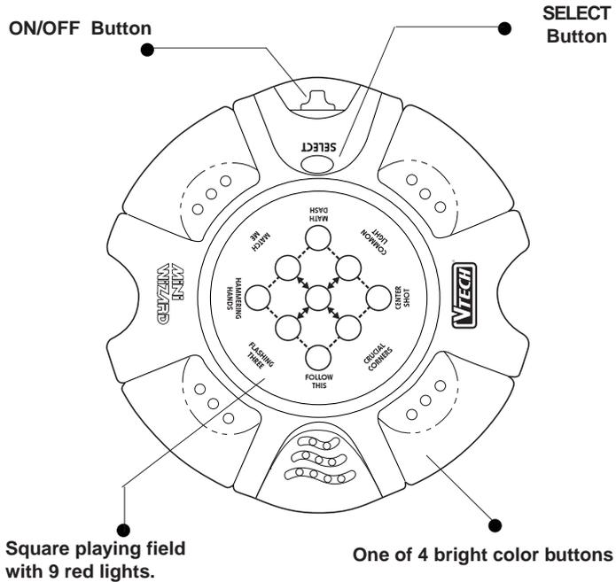
**NOTE:** High/low volume switch is located on the bottom of **MINI WIZARD®**.
