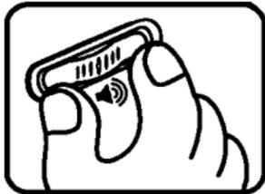
5. To adjust the contrast of the LCD screen, slide the **CONTRAST SWITCH** (
