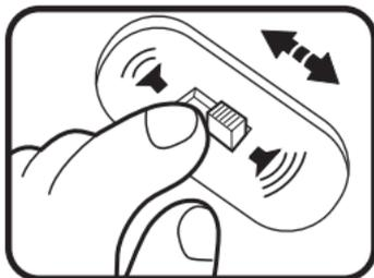
3. Slide the **ON/OFF/MODE SELECTOR SWITCH** to the **OFF** ( ● ) position to turn the unit **OFF**.
