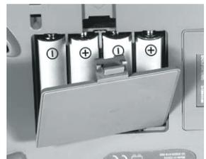
**NOTE:** Replace with new, alkaline batteries.
