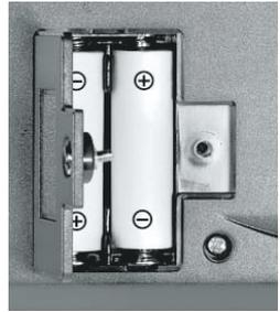
**Important:** While replacing the backup batteries, the 4 “AA” batteries must be kept in the unit or the unit must be plugged into the wall outlet with the adaptor. Otherwise you will lose any information saved on the unit.
