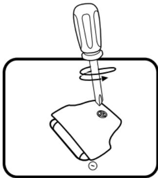
3. Install 1 new AA (AM-3/LR6) battery following the diagram inside the battery box. (The use of a new alkaline battery is recommended for maximum performance.)
