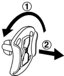
① Rotate the packaging lock counter-clockwise 90 degrees
