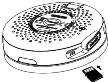
**NOTE: Data stored in the camera's internal memory will not be accessible when a memory card is being used. To prevent accidental data loss, be sure to back up all important data from the camera's internal memory and from your memory card before using it.**
