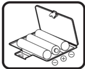
3. Install 3 new "AA" size (LR6/AM-3) batteries following the diagram inside the battery box. (The use of new alkaline batteries is recommended for maximum performance.)
