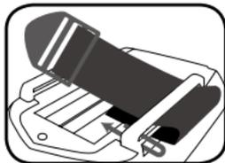
3. Then, pull the end of the tail through the other **Arm Band Slot** and over.
