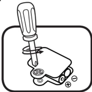
4. Install 2 new AAA (AM-4/LR03) batteries following the diagram inside the battery box. (For best performance, alkaline batteries or fully charged Ni-MH rechargeable batteries are recommended).
