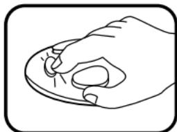
9. Press the **MOUSE EARS** to move the cursor on the LCD screen left or right. Press the left mouse ear to move the cursor left or press the right mouse ear to move the cursor right.
