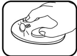
10. Spin the **ROLLER BALL** on the keyboard to move the cursor on the LCD screen up or down. Spin the roller ball up to move the cursor up or spin the roller ball down to move the cursor down.
