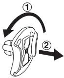
1. Rotate the packaging lock 90 degrees anti-clockwise.
