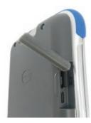
Insert the microSD card with the label side facing down and push until you hear a click.
